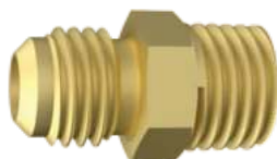
170401 Amarelo NIPLÉ TC X NPT Rosca Externa: TC 3/8" Rosca Externa: NPT 3/8"
